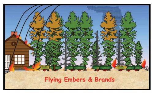
**WIND DRIVEN EMBERS** and firebrands blown ahead of the fire that land in areas that catch or trap them. Heat traps include roof valleys & gutters, open eaves, soffits, overhangs, or under decks and balconies.
