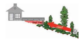
Enclose the underside of balconies and aboveground decks with fire resistant materials.
