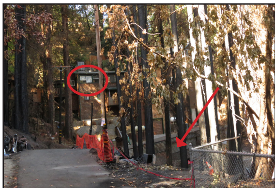
A structure fire at the arrow burned into nearby trees. Radiant heat cracked the window shown in the red circles.
