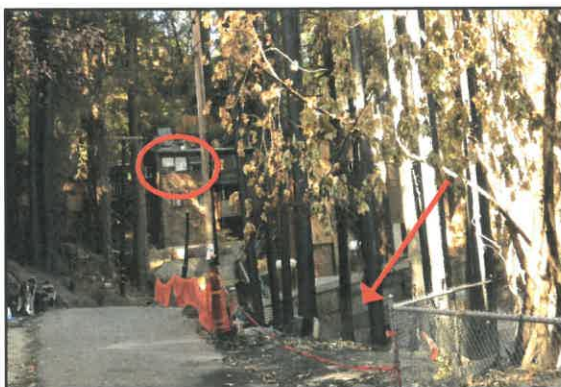
A structure fire at the arrow burned into nearby trees. Radiant heat cracked the window shown in the red circles.
